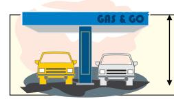
Pump island canopy signs are considered wall signs. For wall signs, the height shall be measured from the base of the building below the sign to the top of the sign face.
