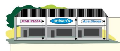
For wall signs, the height shall be measured from the base of the building below the sign to the top of the sign face.
