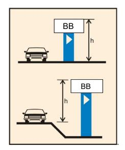
For billboard signs, the height shall be measured from the elevation of the centerline of the adjacent road to the top of the sign.
