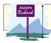
For pylon and ground signs, the height shall be measured from the ground level at the base of the sign to the top edge of the sign.
