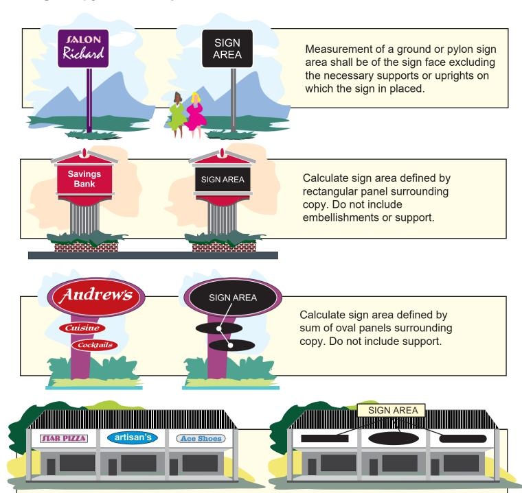
The area of signs which have a face, border or trim shall consist of the entire surface area of the sign on which copy could be placed.
