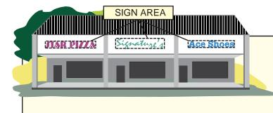
The area of a sign whose message is applied to a background which provides no face, border or trim shall be the area of the smallest rectangle which can encompass emblems and other elements of the sign message.
